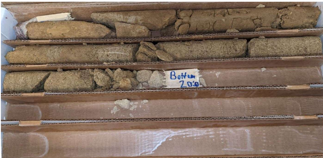
PHOTO 2: Boring B21-31 RC-2 (15.0 - 20.0 feet)
